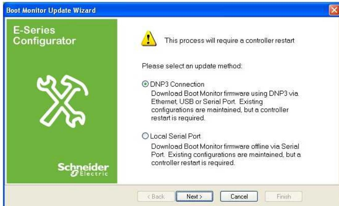
**Figure 7.2: SCADAPack E Configurator Update Boot Monitor Wizard**
